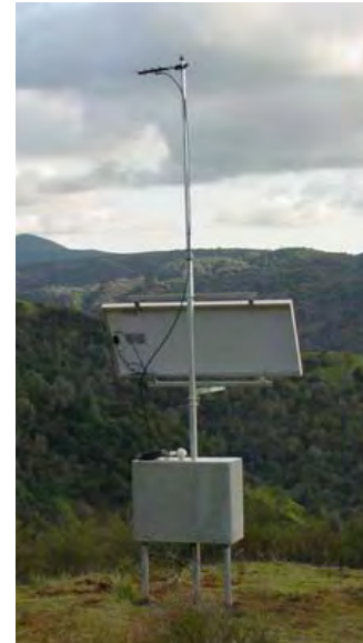
Figure 6 – Schematic diagram of MSA station, including option for telemetry (left) and photo of similar MSA surface installation, showing utility box, solar panel and telemetry antenna (right). Phase I installations at Newberry will not include the mast and antenna above the solar panel.
